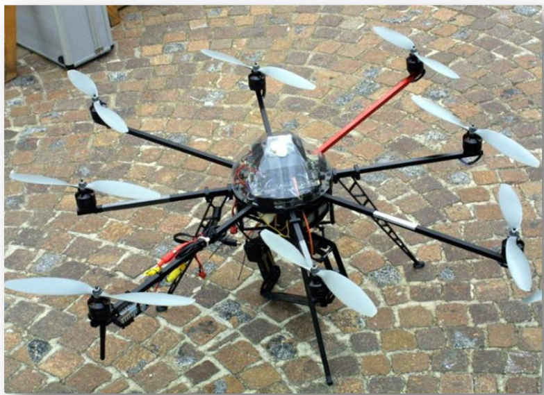
Figure 5. Octocopter used in a real post-seismic scenario. Photo: M. Mormile (2015).
